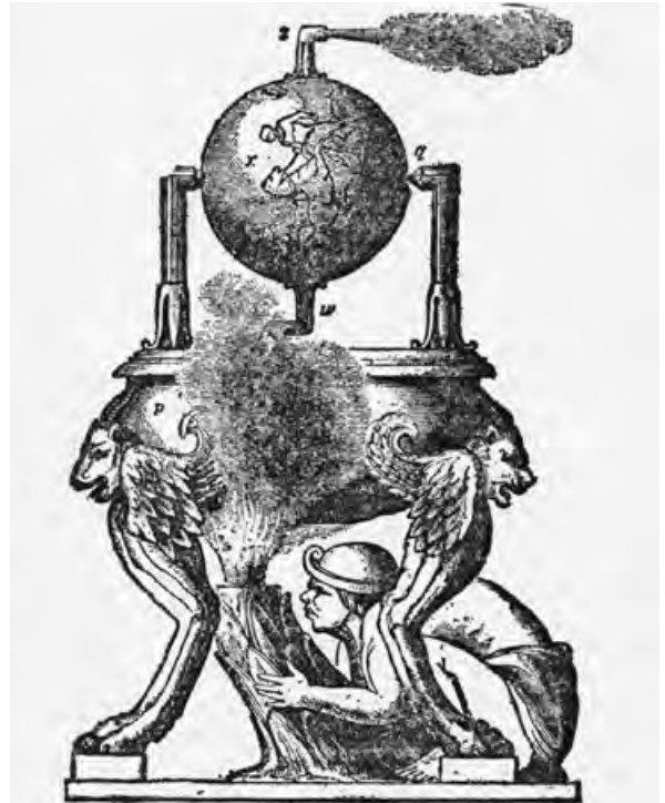
An aeolipile (or aeolipyle, or eolipile), also known as a Hero engine, is a rocket style jet engine which spins when heated. In the 1 st century CE, Hero of Alexandria described the device, and many sources give him the credit for its invention.
